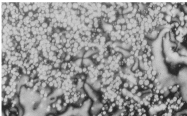
Fig. 7 - The droplets formed on cooling the isotropic liquid of the copolymer prepared from (R)-[SO] and the racemic oxirane with the -\text{CH}_2\text{-O-(CH}_2)_6\text{-} spacer
